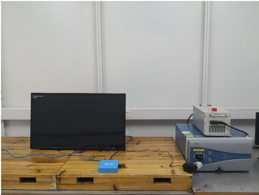
EFT SURGE and DIPS IMMUNITY TEST SETUP-AC POWER PORT
