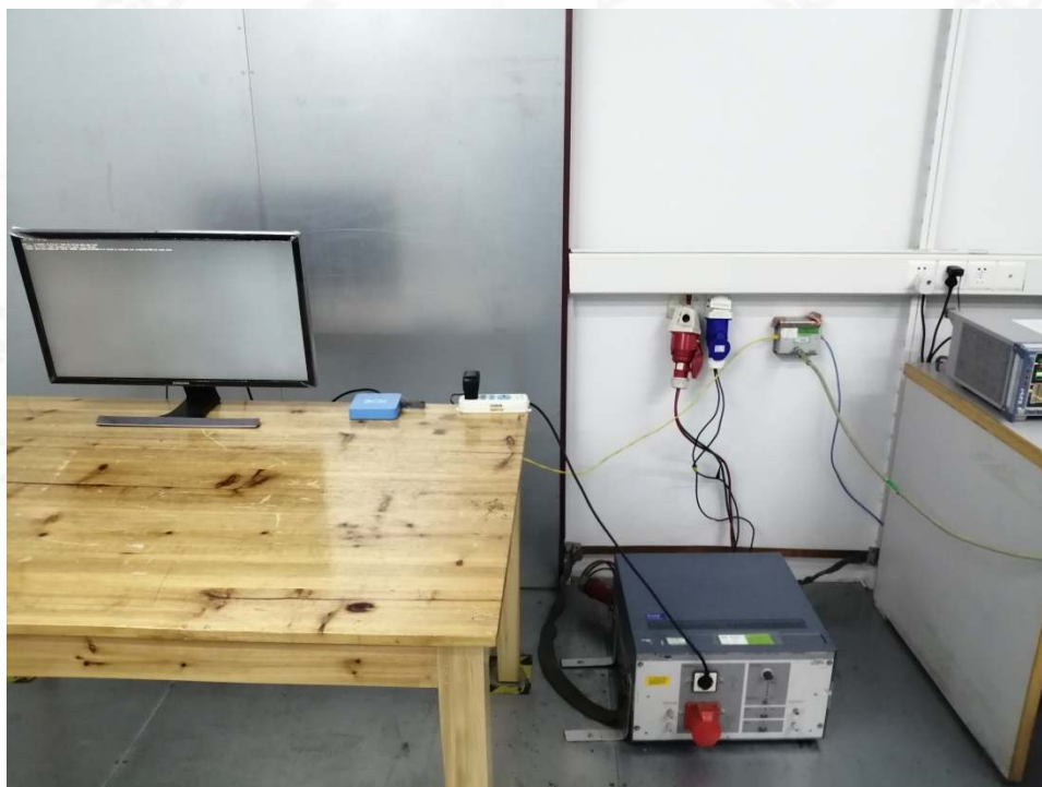
EN 55032 CONDUCTED EMISSION TEST SETUP (LAN)
