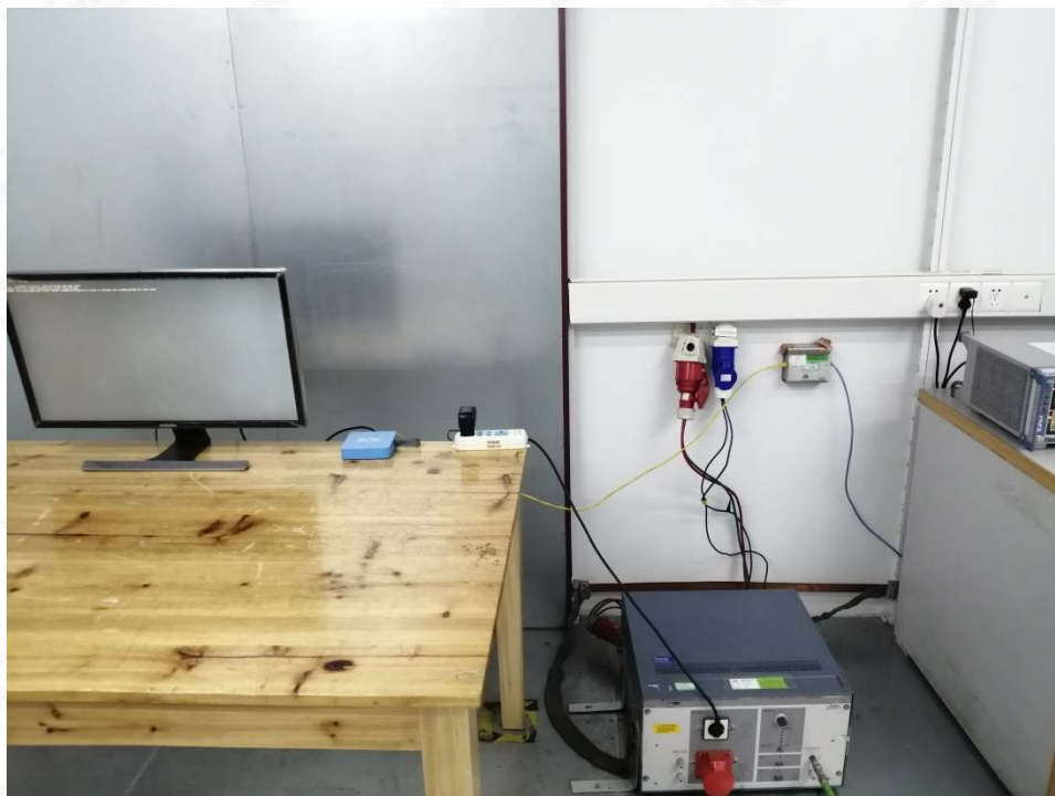
EN 55032 CONDUCTED EMISSION TEST SETUP (LAN)
